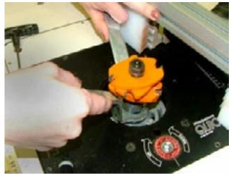
Andrea will be setting this bit up to cut 5mm thick tenons. She wants to shape stave ends to fit mortises that are cut with the Festool Domino Joiner. She uses a 5mm thick Domino tenon to serve as a setup gauge.
