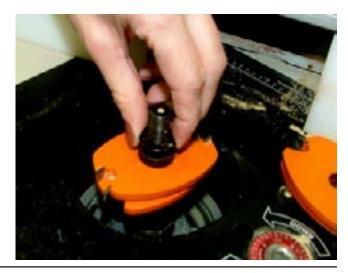
The adjustment works. She has a tenon that is just the right thickness. Now, she can make wider mortises or use a hand saw to trim the tenon width. The hard part is done. The tenon fits well and she now can record the combination of spacers that will allow her to replicate the 5mm tenon at any time.
