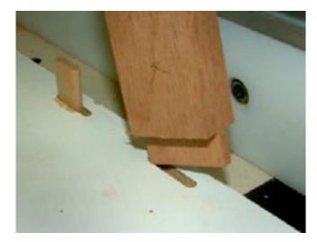
Andrea is proud of her new found skill. The CMT Tenon Cutter is a precision tool that allows precision cuts. It can produce tenons with thicknesses between the 3/16" and 3/8" shown above — and in metric as well.
