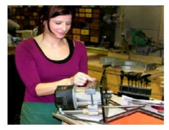
The round body of the router fits into the lift's cradle and is quickly locked in place.
