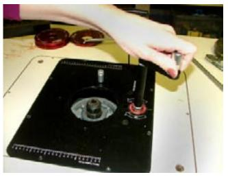
This is the product shot from Woodpeckers website. I show it because it displays the other way to adjust the height of the router. The steel L-handle device is inserted and then turned 1/4 turn to allow the router to be brought up or down quickly. It is a nice picture isn't it?
