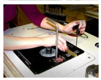
She takes a few minutes to adjust the insert height so that the top is in perfect alignment with the router table top.
