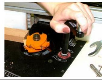
Just as she would when cutting a coped end of a rail, Andrea runs the sample through the cutter using a square scrap of MDF to serve as a backer board and help her keep the sample square to the fence.
