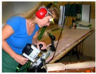
The CMT Tenon Cutter set makes matching the tenon width to the mortise a relatively easy task. It is just a matter of removing or adding a combination of spacers.
