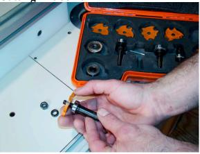
Set up your slot cutter. Secure it in the router.
