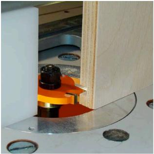
**Reset the height of the bit** for the next cut. Make the top of the bit even with the bottom of the groove. It's best if you don't disturb the fence position. That way the depth of the groove and the length of the tongue will be the same.
