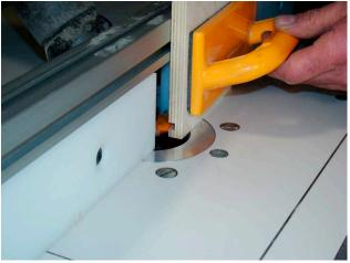
Make a test cut. After the test cut, reset the bit height and fence position as needed, then machine grooves into the ends of the drawer sides.
