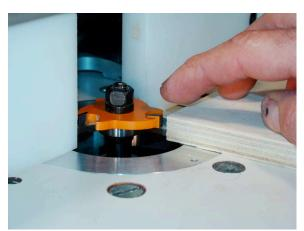
Set the height of the cutter. The top of the bit should be even with or slightly above the top face of the material
