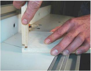
**Test the fit.** If the joint is too loose lower the bit to make the tongue larger. If the joint is too tight raise the bit to make the tongue smaller.
