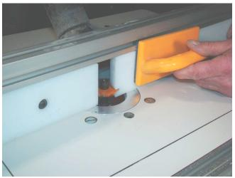
If there is excessive chipping on the inside face of the sides, **cut a zero clearance fence** on the infeed side of your router table fence
