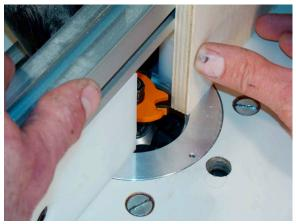
**Position the fence.** Set the fence so the bit will cut into the material by 1/2 the material thickness.
