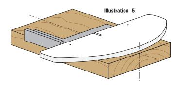
**NOTE:** DRIVE NAILS IN ABOUT 1/4"-3/8" (6,35-9,5mm). THE NAIL HOLES WILL BE MACHINED OUT WHEN RAISED PANEL CUT IS MADE.
