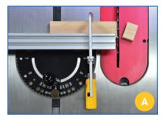
Clamp a piece of scrap to the miter gauge. Trim off the edge with the blade you will be using for your crosscut dado.
