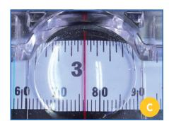
Leg #1 of the Dado Stop is exactly 3" in length. Set your rip fence scale cursor to exactly 3". Now your fence gauge will read accurately for this blade.
