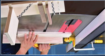
Effortlessly cut exact dado width using a standard table saw blade.
