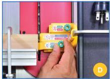
Adjust Leg #2 in front of the blade until touching the edge of the scrap trimmed earlier.
