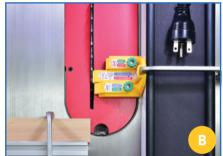
Unplug the saw. Attach the Dado Stop to your rip fence using a MATCHFIT Dovetail Clamp. Adjust the rip fence so Leg #1 is gently touching the right side of the carbide teeth at the front of the saw blade.
