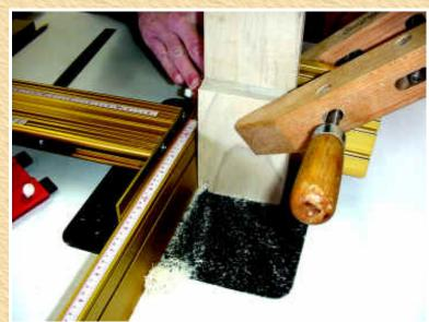
Here I am making my first cut. I have clamped the two end pieces together with a backer board. I used a wood clamp to secure these pieces to the right angle fixture. The backer board is a scrap piece that will minimize tearout.
