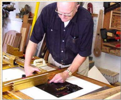
To set the fence properly, I first move it until the router bit is centered at the edge of the fence. This is what it looks like:
