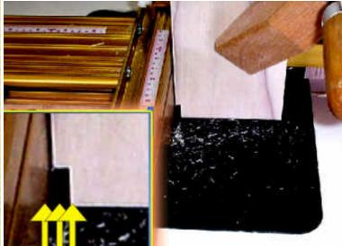
For the outside cuts, the instructions suggest "sneaking up" on this cut by making several light passes before the actual first full "B" cut. This minimizes splintering of the ends.
