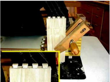
When done on one end, I flip the boards end-for-end and make the cuts on the other end. The inset shows you the already completed ends with the rabbets. The end pieces get the "A" cuts. The Incra Stop (red part) is placed on the fence and adjusted so that the stop is as close to the bit as is possible. The cuts are made with the piece laying flat on the table and against the fence using a push block. The stop limits the depth of cut.
