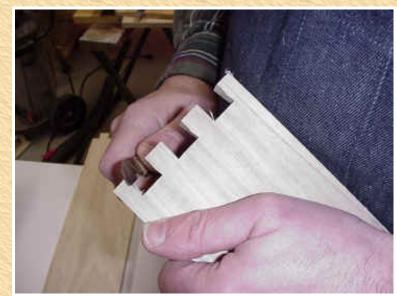
The third cut is simply to remove a tiny nib that is left from the first two cuts. I used a chip carving knife to remove it in one simple stroke. Absolutely no carving skill is required. A chisel or utility knife could be as easily used.
