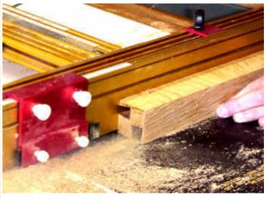
Once the straight bit has done its job, I install the dovetail bit again and make a pass. Even in this very dense quarter-sawn oak, the dovetail bit makes an easy cut, now that the straight bit removed the bulk of the slot. Now it is time to cut the sides.
