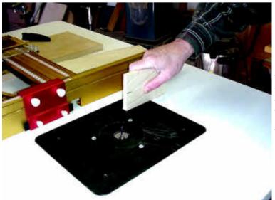
Before I go further, I use a block of wood to be sure that the router plate insert is absolutely level with the table. I do not want even the smallest bit of unevenness when sliding the right angle fixture and wood pieces back and forth. The Woodhaven router table has an excellent leveling adjustment system that makes this very possible.
