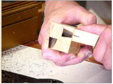
Now you can see that the dovetail marking is a good way to show where the actual dovetails will be. I position the side piece, with the centerline marked, to see if the reveal is correct. It looks good. It is time to cut the legs. I set the Incra Stop to cut the groove the width of the side, less about 3/8". This can be approximate since we will trim the tails to fit. Once set, I move the Incra Stop's scale to 0°, so that I can remove the Incra Stop and later return it to the exact position.
