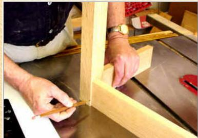
This is a sample of the leg/apron joint I will use. The oak leg measures 1 3/4" square, and I have cut sample apron pieces of 3/4" oak stock in a 3" width.
