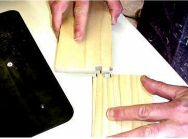
Then you flip one board over and put the two together. If they fit perfectly, your router depth is set exactly right.
