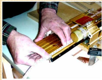
And slide the template into one of the jig's tracks. There are several tracks on the Ultra. It doesn't matter which one you use. At this point, I slide it all the way in; I will position it exactly in one of the next steps.
