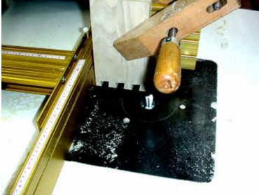
The end board pins are cut in three steps: the first step is to cut the pins exactly like the sides (tails) were cut but using the "B" settings.
