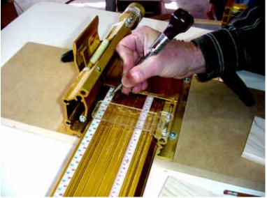
With the fence carriage locked, I move the template so that the "center mark" is directly under the alignment line. The long strip can be difficult to move so I used an awl to budge it. Be careful not to mar the template or carriage. The "center mark" can be any of the marks but there is a
