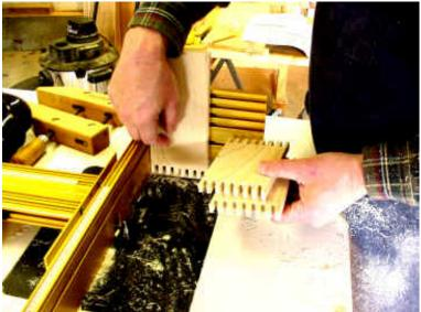
The two end pieces are done with the "A" cuts. You can see the backer board still in place on the right angle fixture. I have flipped the backer board and am placing the sides in position to receive the "B" cuts.
