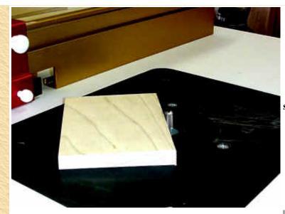
Since this is a box joint, I adjust the router depth to a slightly greater depth than the thickness of my stock.
