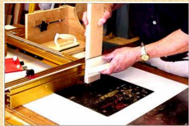
I have two sample side pieces. The first step is to rabbet the ends using the very same dovetail bit at the very same height. I have started by placing the fence 1/16" in. I will cut one side and then the other, and then check the fit. You can use a simple push block like this.
