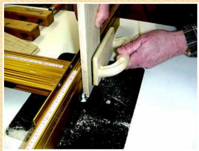
The instructions say to cut "a dovetail shaped rabbet" in both ends of the pin (end) boards. The template tells you how deep this rabbet should be and the guide helps you set it. You make this cut on one side and on both ends of the front and back pieces.
