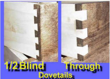
Now the "through dovetails." I must say that I had real trepidation about making these on this jig. For one, I didn't know how a single dovetail bit could cut both tails and pins. After all, the jigs I have experience with used a dovetail bit and a straight bit. Reading the instructions, at first, didn't help. "Whittling" as the last step seemed to defeat the purpose of such a precision jig. Maybe this jig really isn't meant for this joint.
