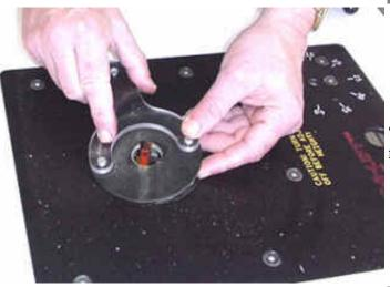
I install as small an insert plate that the bit will allow. The Rout-R-Lift insert plates are nicely machined and fasten in place easily and positively.
