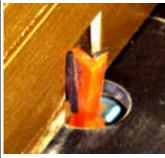
With the fence centered over the dovetail bit, I move the template to read "0" under the cursor. In this photo, I am using the middle scale. The upper scale is set for measuring distance to the saw blade when the unit is shifted to the table saw position. The lower scale is a centering scale used in drawer dovetailing and other operations.
