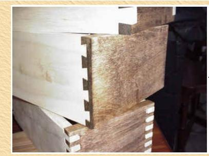
While I stained the end so that the joint would photograph better, I didn't have to sand either piece. The joint was absolutely tight fitting...a very nice half-blind dovetail.
