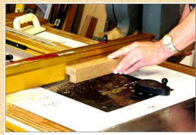
The leg is white oak and very dense. There is no way that I can make a cut with a dovetail bit without first removing as much of the groove as possible.
