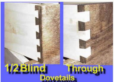
With the box joint accomplished, I am ready to try dovetails. The Incra Jig can do both half-blind and through dovetails and while I am wanting to do the latter for my chest project (I am adding special drawer fronts to the drawer boxes), I decided to learn to do half-blind dovetails first.
