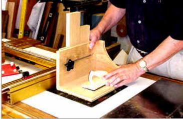
I think this is proof that the jig controls the cutting much better and it can handle two boards at a time. After rabbeting both sides at 1/16", I test fit the tail. It is too big. I visually check to see how much there is to remove. I do not want to go over and have too small a tail.
