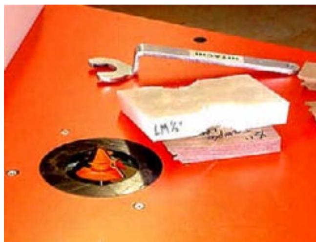
As I do every time that I put an insert in the fence, I first check to see that it clears the stopped cutter. Then, while standing behind the fence, I turn on the router and move the fence cautiously over the router. That serves to cut any minor discrepancies of the bit setup and is a good safety procedure.
