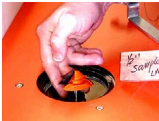
Having a sample block does make the set up of any bit very fast and accurate. From this view, you can see that the bit height is not left to guess work or trail and error. It can be very exact.
