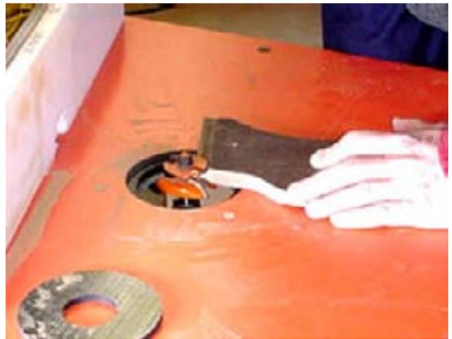
I have lowered the router speed. This is a 2 1/2” bit and the maximum speed for that diameter is 16,000.
