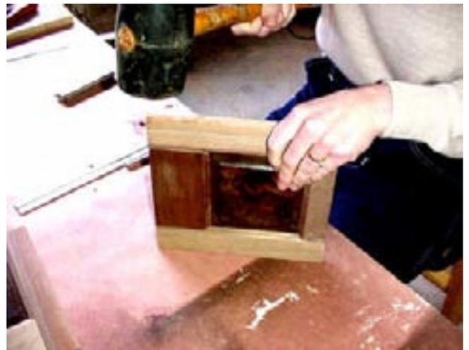
She places the side panel in the clamps to dry. Note that she has a front panel clamped as well. This is not glued at this point. It is in the clamp to mate with the locking miter corner to keep the corner from being crushed by the clamp.
