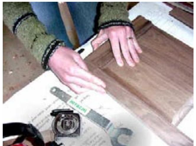
Beth picks up where she left off last week. The back panel has been glued up. The two raised panels have been inserted in the rail and stile groove. The top panel is a piece of 1/4" veneered plywood. It will be added when the other veneered pieces and the glass are added.
