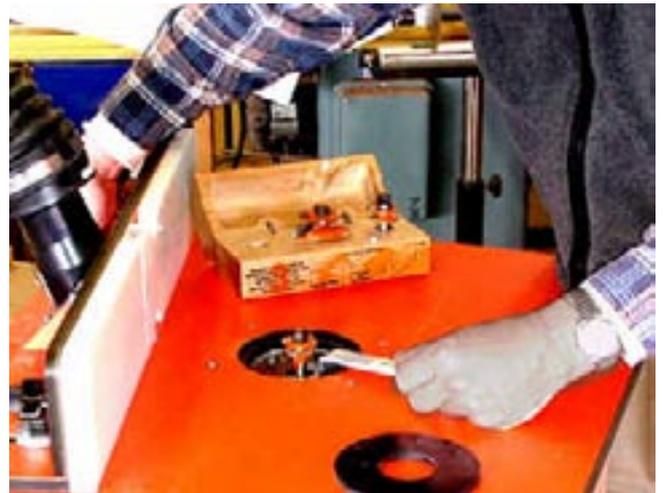
I have said many times, that I love the bent wrench. I realize that what I haven't mentioned is that the Hitachi M12V collet is amazing. It takes less than a 1/4-turn to lock and unlock the collet. Every other router I own takes one or more turns. This setup I have makes changing bits amazingly quick and easy.
