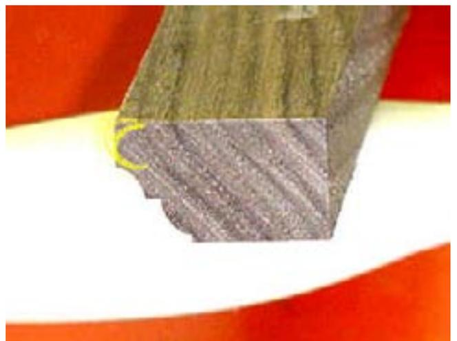
I make the second, rounding over pass using just this one section of the multi-profile bits. I have several of those and it always amazes me when I can make use of just a bit of it. It saves the day this time.
