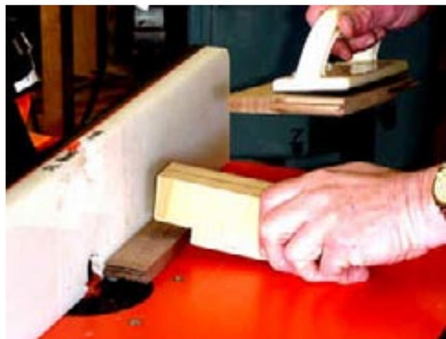
Here I am running the stock. My left hand keeps pressure on the piece so that it is on the table and against the fence. My right hand is using the MDF pushblock to push the piece through the cutter.
