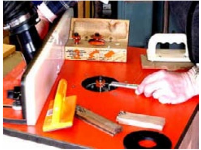
I use the sample piece to double-check the height. When the router bit is rotated, the cutter should just “kiss” the groove of the sample. It does.
