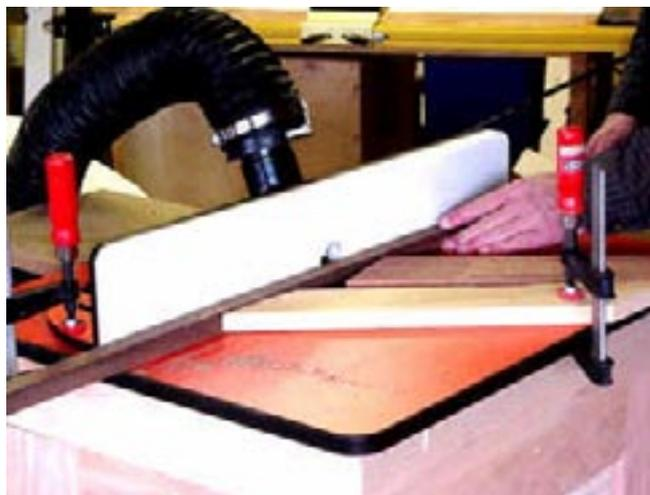
Several router passes later and you can see what the outside molding looks like. The two edges have a slight ogee shape, and I am now rounding over the outside corner. The trick to making moldings is to set up each cut with sufficient hold downs or to use push blocks. The smoother the routing, the less follow-up sanding is required.
