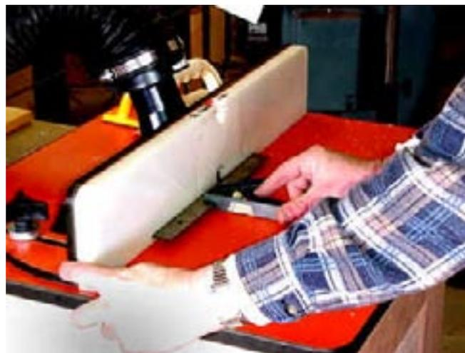
The rails and stiles will be profiled along their length. The narrow stiles can be run by using the push block with the MDF. By rotating it 90o, a fresh edge can be used to push the through the cutter.
