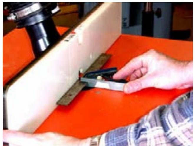
The fence is used to guide the ends of the rails. I have added a new piece of MDF to the push block. This will serve as a backer board and will keep the rail perpendicular to the fence.
