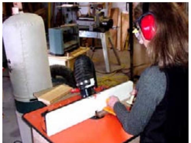
With the ends of the rails coped, Beth attaches one of the templates to a rail piece which will be shaped with the graceful crown at the top of the clock.
