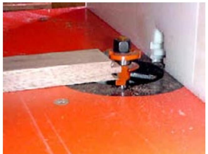
Lastly, she adjusts the fence using the straight edge to align the fence with the pattern bearing.
