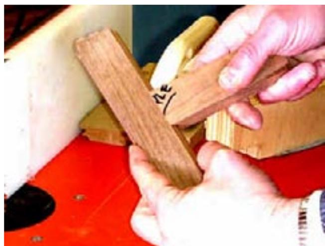
For the wider rails, I switch back to the standard pushblock.
