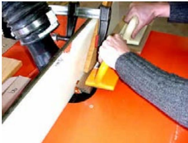
She runs the mating piece against the fence. The walnut mills very well. While the fence was set to make the final cut in one pass, she makes a second pass just to “clean out” the cut.
