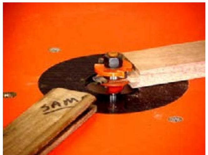
Now, I install the fence insert with the shape cut-out for that bit. Having marked the top helps to identify the correct insert.
