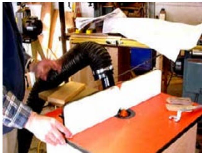
When the router comes to a complete stop, I move the fence into the bit and use the sample cut to adjust the fence depth.
