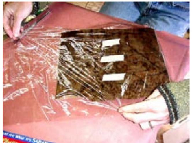
She has placed the plastic wrapped sandwich on the trim board and is now placing the top in position. These boards will help spread the clamping pressure uniformly on the veneer sides.
