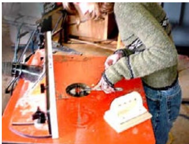
Having placed the sample on the infeed side, Beth has installed two feather boards. One is clamped to the fence and holds the piece down on the table. She is clamping the second to the table having positioned it to hold the piece tight against the fence.
