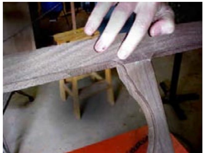
he starts by using a straight edge and knife to score a straight line using the straight part of the rabbet as a guide.
