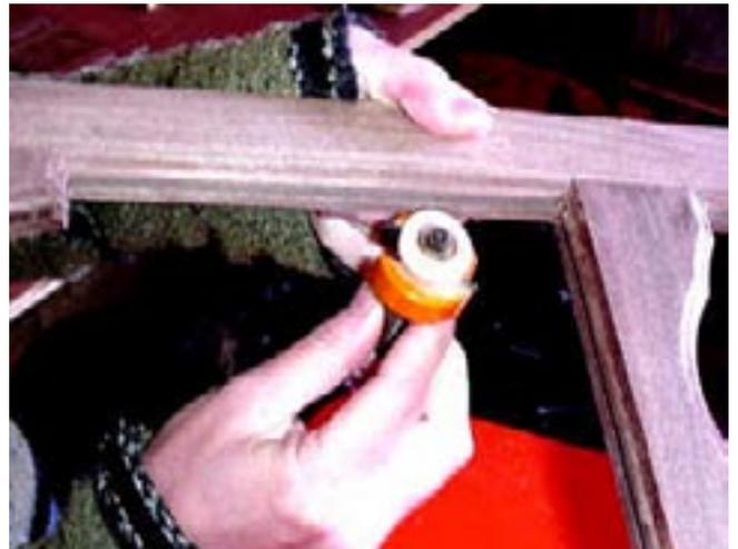
Beth adjusts the router height until the bearing rides against the molding edge.
