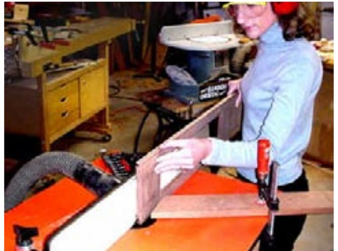
With the grooves cut in the sides, Beth now installs the other cutter. This one will be adjusted so that it cuts a tongue that is centered on the 1/2" frame stock.
