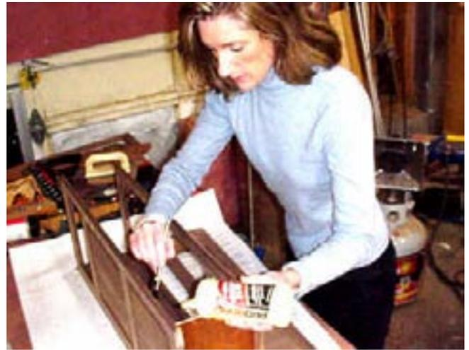
With the glue spread, she adds the side and turns the assembly over to glue the other side.
