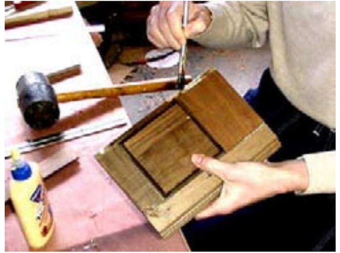
She carefully taps the stile back onto the assembly. She then flips it around and removes the other stile, glues and reassembles. Not only does this keep all the parts in order, but it is much easier to manage.
