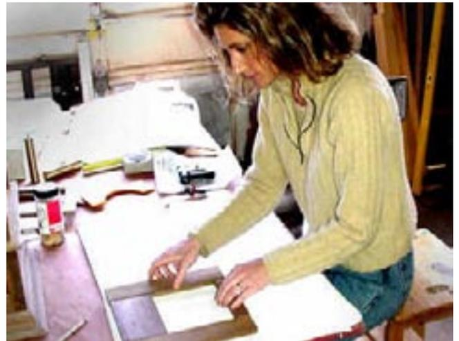
The plans say to glue up the frame and then use the template for shaping the upper rail. While that will give us a larger piece to hold when routing, we decided that we should make the rough cut at the bandsaw before we glue the pieces together. Of course we could use a saber saw to make the rough cut after the glueup.
