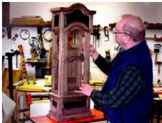
Last week, Beth and I added the molding around the base and top units. What I forgot is that there is also a piece of molding that covers the butt joints of the sides and front.
