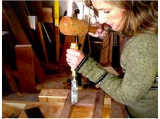
With the bulk of the material removed, she uses hand pressure to shear the rabbet walls smooth.
