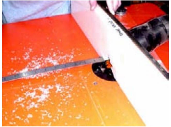
Beth has clamped a featherboard in place to keep pressure on the side as it is routed.
