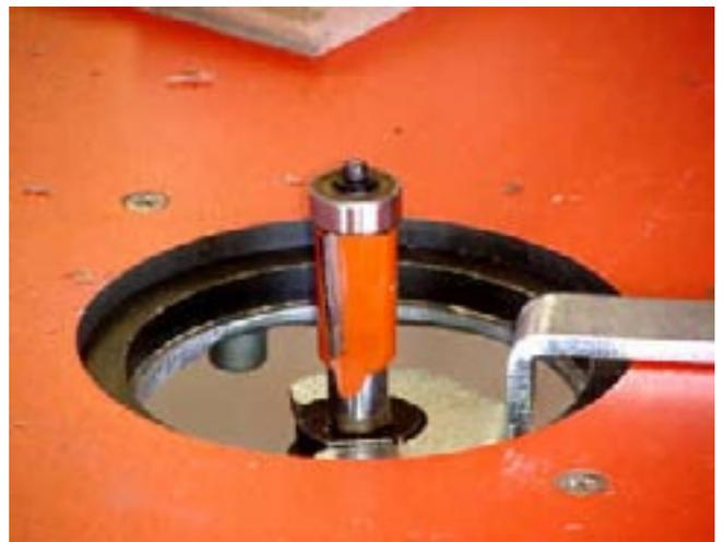
As you could see in the first picture, above, this template has extensions on both ends that protrude beyond the workpiece. These allow you to start the shaping at the left end (near) with the cutter not contacting the wood. With the bearing firm on the extension, you can move the piece and have a smooth, controlled start.
