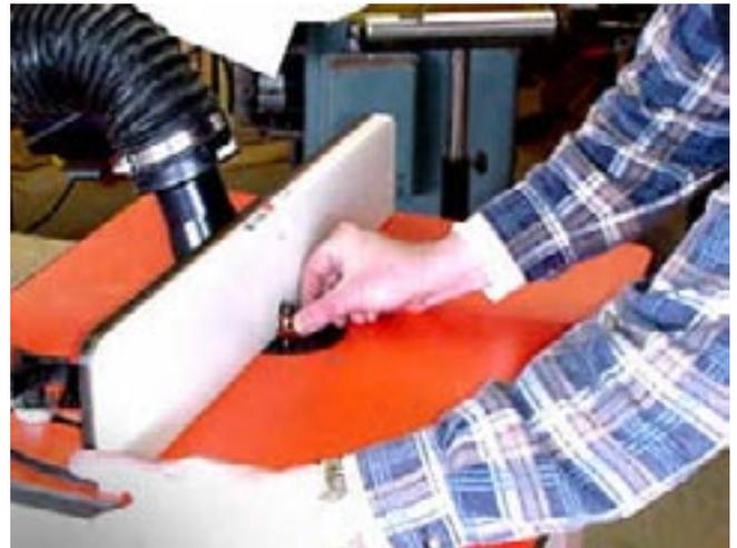
Then, standing behind the fence, I turn the router on and move the fence carefully over the bit. This is a safety precaution to ensure that the bit will rotate smoothly when in the insert. I then turn off the router and let the bit come to a complete stop.
