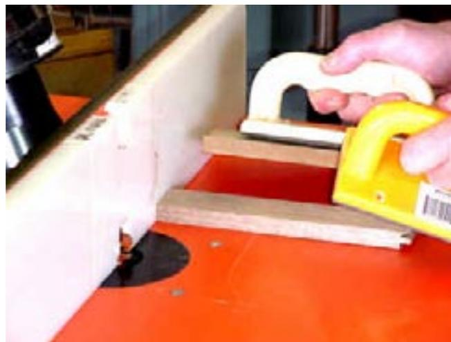
A second push block allows me to use my left hand to hold the rail against the MDF-pushblock and the fence and flat on the table. The right hand does the pushing of the rail through the cutter. The customized, zero-clearance, insert keeps the stock from “dipping” into the space around the bit.
