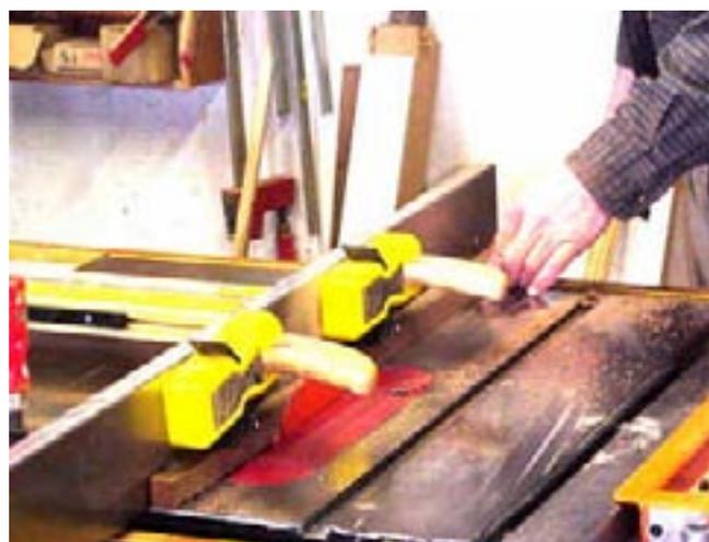
At the router, I make several passes with the rabbeting bit. This piece will be an outside corner molding so I want to rabbet the inside to leave 1/4" sides. The two finger boards help to keep the stock square against the fence.
