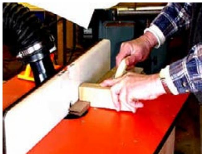
I check the fit using the sample block. It is perfect, so I can run all the stiles and rails.
