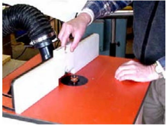
I move the fence forward to see that the bit does, in fact, clear the opening as I manually rotate the bit.
