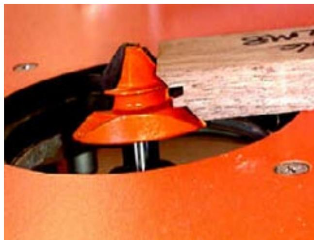
I store the sample cut with the fence insert for that bit. This insert happens to have two profiles cut in it. One is for this bit in 1/2" stock and the other for 3/4" stock. Labeling helps to keep the inserts straight.
