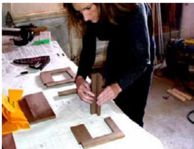
It is time to cut the cope ends on all the rails of the sides and the front panel. She selects the cope cutter – it is the one with the bearing in the middle.
