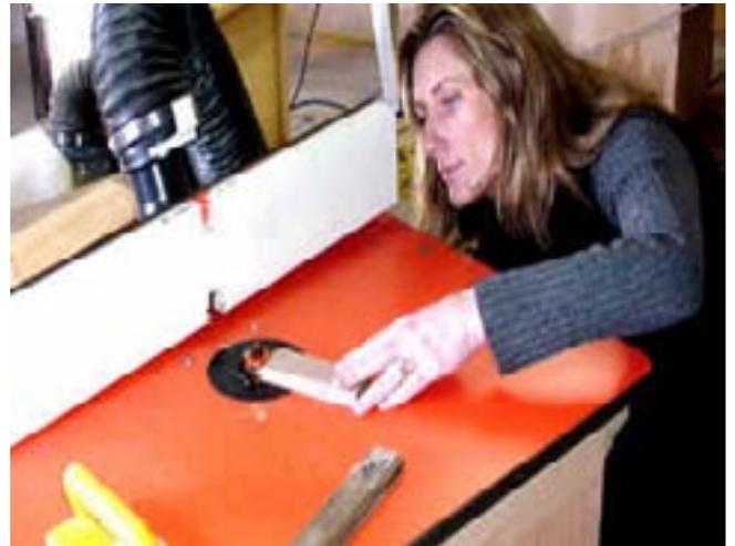
She slides the insert that is cut for that profile. Each fence insert is labeled with the profile.
