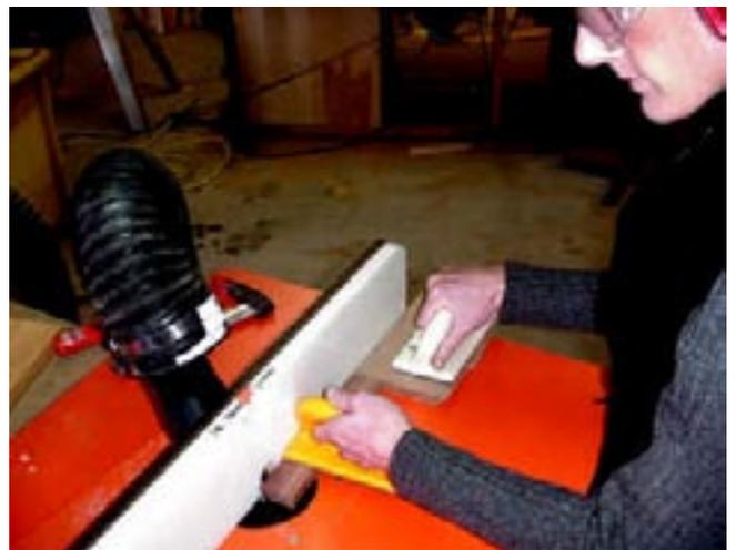
It has taken Beth very little time to make the cuts using the CMT/Sommerfeld Junior Raised Panel Set. The two profile bits are matched so that once you have one set to the correct height, the other bit can be used without resetting the router height. This feature is also a feature of the standard raised panel set and really makes using these cutters easy.
