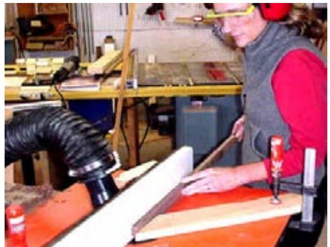
It is funny how coming back to a problem another day can make the problem go away. I used a classic bit on the base piece that is now installed. The piece I am now marking was cut with another ogee cutter using only a portion of the profile.
