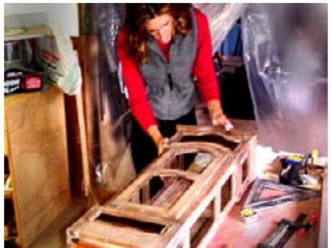
Beth and I have been sanding each piece at every step of the way. She uses the orbital sander and 220 grit paper to remove a few glue marks. She is using the orange pad to keep the sander away from the finished raised panel – it would not be good to scratch these veneered surfaces that we have labored over.
