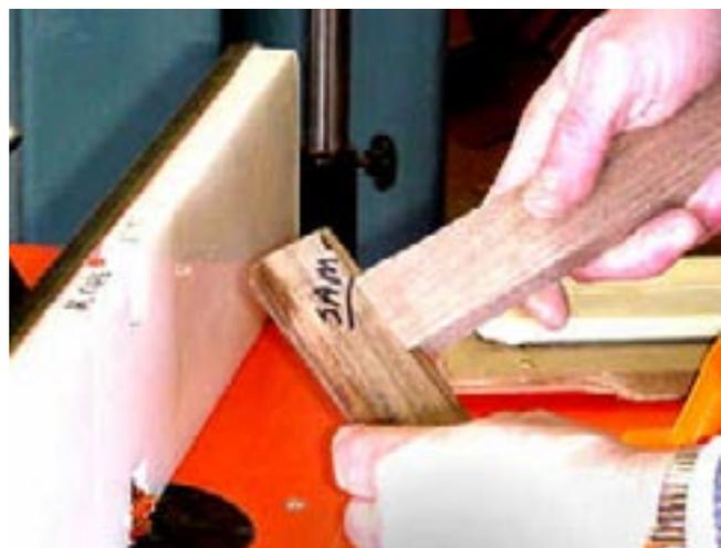
With the rail ends coped, we can change bits and cut the profile on the rails and stiles that will accommodate the raised panel.
