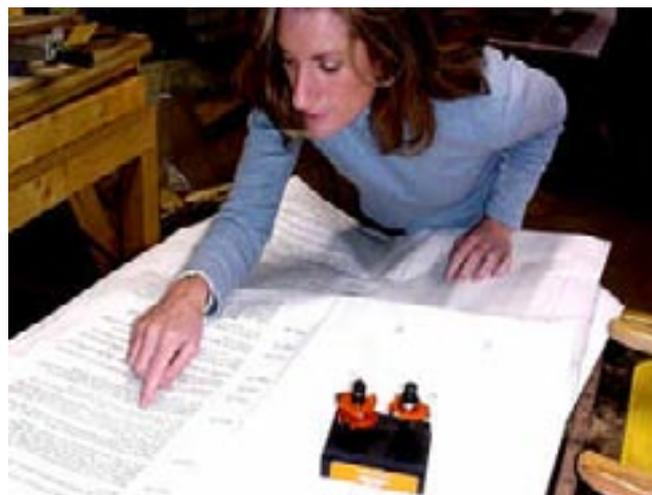
Two grooves will be cut into the length of both sides. The tongue is designed to cut a 1/4” width. The bearing allows a 3/8” depth of cut – much too much for 1/2” stock. The plans explain how to swap the pattern bearing to make a 1/4” cut. Rather than to change bearings, Beth and I decide that we can use the fence to limit this depth.
