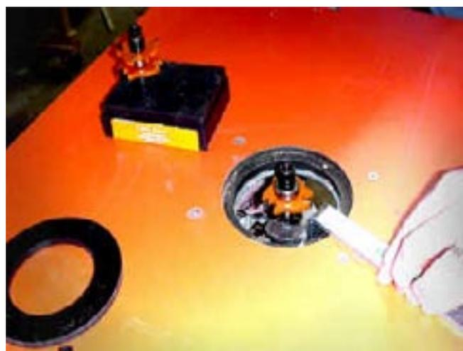
Beth adjusts the fence so that the cutter depth is 1/4". She has raised the router so that the cutter is 1/8" above the table.
