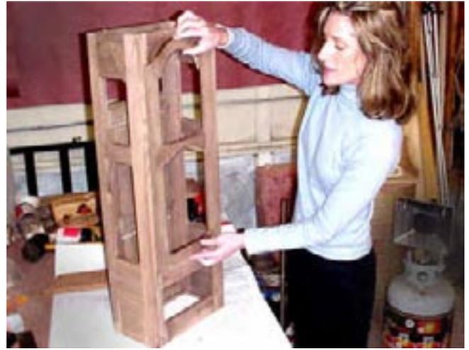
She has cut a spare piece of 1/4" plywood to fit loosely in the floor groove she just cut.
