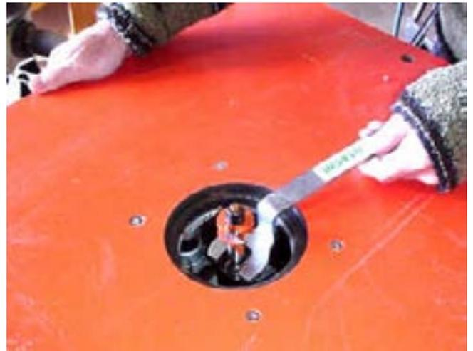
She installs the fence insert that has been cut for this bit.
