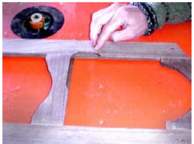
She determines that the rabbet should be slightly deeper, so she changes the pattern bearing. The bearing set at the left allows her to adjust the rabbet depth by swapping bearings. This assortment of bearing is very handy for use with a lot of pattern bearing bits.
