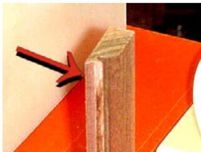
On the other hand, when you are running the stock and you see a slight gap on the outfeed side of the fence, the fence should be adjusted in until it touches the stock.
