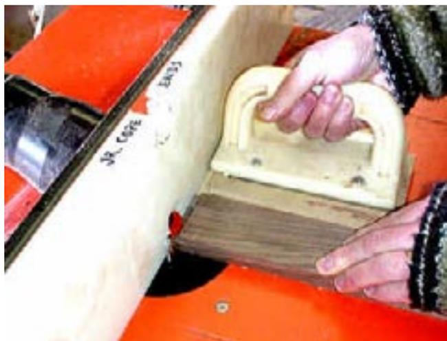
With the fence backed away and the insert removed, Beth changes the bit to the rail and stile profiling bit. Since it is a part of a matched set, the height should be right without any new adjustment. She checks it with the sample. It is. With this cutter's fence insert installed, she brings the fence up to the bearing, and she is ready to go.
