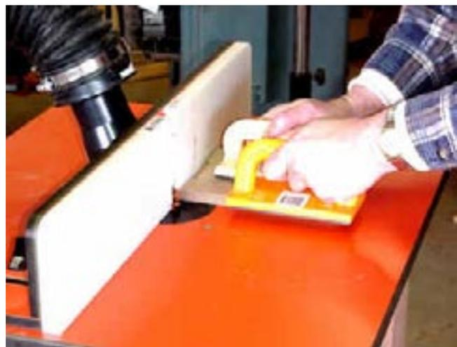
I test fit this newly cut rail to my sample piece. It fits perfectly, so I can make all the cuts on both ends of each of the rail pieces.
