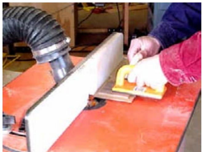
I said a minute ago that you want to shape the ends of the curved panel. Here is why. In the picture at the right, I have moved the workpiece against the cutter's bearing. Since this short edge was routed in the last step, I can safely ease the workpiece onto the bearing at this pre-shaped location.
