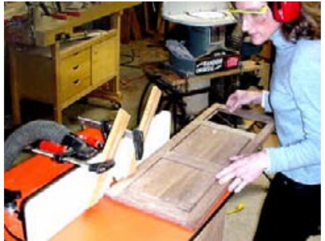
The next step, is to cut a dado across all the panels to hold a floor in place. We were concerned that the dado would show through at the corners, but a search of the plans showed us that it would be covered by the base unit.
