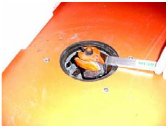
While we had used the other two cutters before, we had not used the raised panel cutter with the new Sommerfeld fence. Beth is marking a new insert with the profile of this bit.
