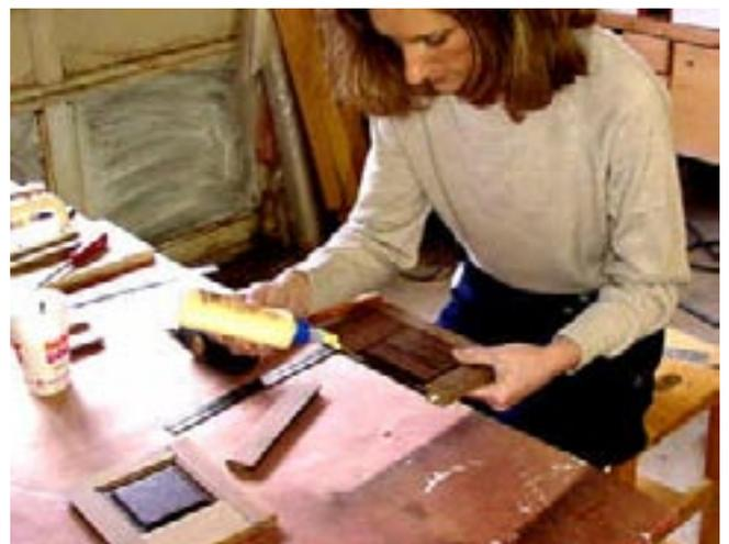
She carefully brushes the glue into the coped area being careful not to spread any in the panel section.
