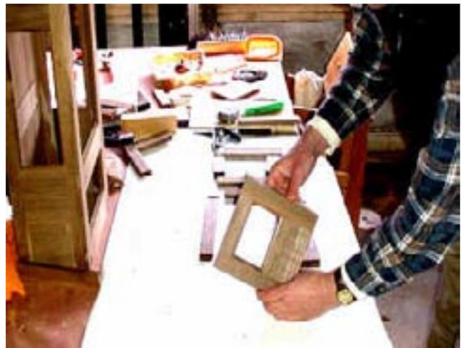
I am only dry fitting at this point and want to give you an idea of how the sections go together. The locking miter joint, we did first, will be the corner post. [Note, the gap at the corner is because I am not holding the corner together.]
