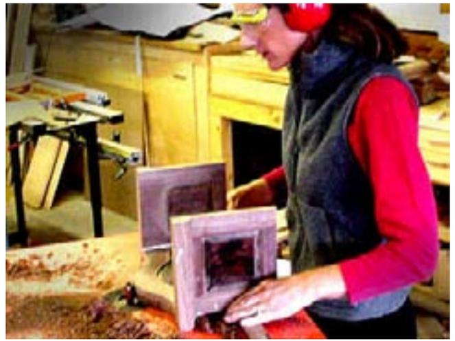
This close-up give a much better view of this operation. The bearing of the trim bit simply follows the shape of the top assembly – a very smooth and safe cut that matches exactly.
