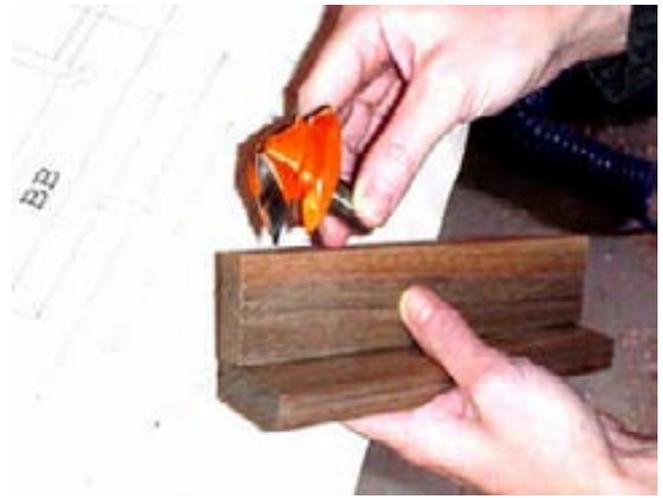
She is using the bent wrench to install the bit in the router. She has already put the fence insert in place for this bit.
