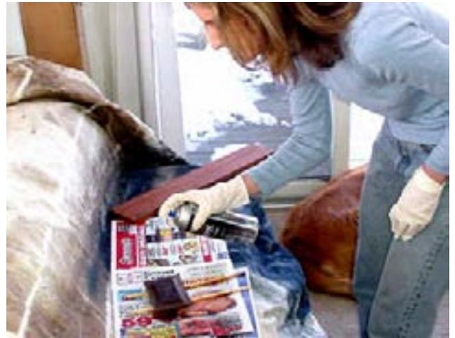
In between coats of the polyurethane, Beth sands the veneered, flat areas with a sanding block and 220 grit paper. She follows this with a piece of the paper rolled up to smooth the MDF edges.
