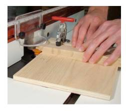
Allowing the bearing on the cope cutter to ride on the base of the sled, under cut the tenon and cope both ends of the rails.
