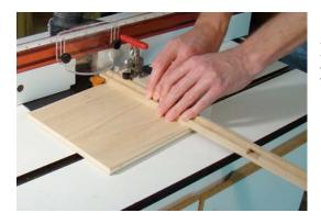
Position the mullions in the sled the same way you positioned the rails and cope both ends.
