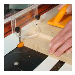
Complete the tenons on both ends of the rails and mullions and on one end of the muntins. Do not tenon the second end of the muntins at this time.
