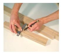
Lay out the location of the mullion mortises on the rails. The mortises should be as long as the mullions are wide, 7/8-in.
