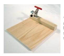
This sled is used to cope the ends of the rails, muntins, and mullions. The plywood base should be 1/2-in. thick. The backer board should be 7/8-in. thick. The toggle clamp used to secure the material is available at woodworking specialty stores.
