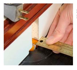
Reset the fence position to cut a 1/8-in. rabbet. Do not change the height of the bit.
