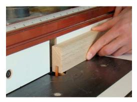
Using the router table fence, center the bit on your stock. Finish the mortises on the stiles.
