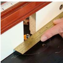
Position the fence by aligning the face of the fence with the ball bearing on the bit.
