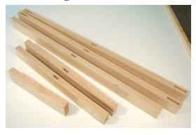
Cut 1/4-in. mortises 1-1/16-in. deep. The mortises are located 5/16-in. from the face of the board. If you've correctly machined your stock to 7/8-in. thick, this centers the mortise. If you cut the mortises using a router you'll need to square the ends of each mortise. Cut the stiles to finished length. The board with no mortises is for the two muntins.
