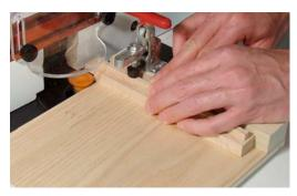
Position the muntins in the sled and cope <u>the</u> <u>tenon end only</u> using the same positioning as the mullion and rails.
