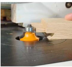
Set the height of the bit so the top corner of the bit is even with the bottom face of the tenon.
