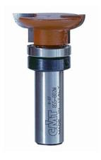
Install the cope cutter in the router table.
