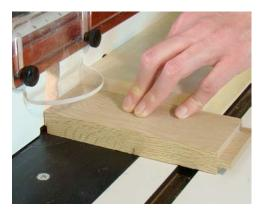
After cutting the piece to length cut a small rabbet on the <u>bottom only</u> of the piece.
