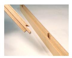
The vertical mullion is joined to the rails with a simple mortise and tenon. The horizontal muntins are joined to the stiles with the same joint.
