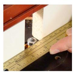
Make the face of the fence even with the ball bearing on the bit.
