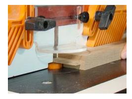
Without changing the height of the bit or the fence position, cut rabbets on the inside back edge of the rails and stiles.
