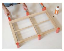
Assemble your door. Because of the number of pieces involved you may find it easiest to assemble sub-sections first. For example, glue and clamp the rails and mullion, allow to dry, then assemble the rest of the door.
