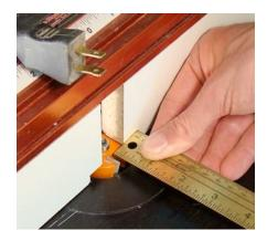
Reset the fence position for a 5/16-in. rabbet. Do not change the height of the bit.
