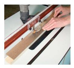
Machine the muntins and mullion to final width. Using the narrow parts sled cut rabbets in both bottom edges of each piece.
