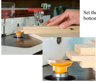
Set the height of the cutter so it just skims the bottom of the tenon.
