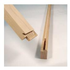
The rails are joined to the stiles with a haunched mortise and tenon joint. You can cut the mortises in the stiles using a mortiser or router. The tenons on the rails are made using the rabbet bit included in the set.
