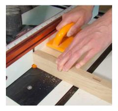
Cut haunches on the rails only. With the rails' outside edge down on the table, cut the haunches first. Use a backer board to reduce tear out. Make the opening in the fence as narrow as possible.
