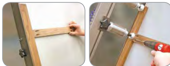
Flush Face Frames Made Easy: 1) Align stile and rail along squaring fence 2) Adjust clamp cylinder and secure joint line 3) Drive self-tapping screw
