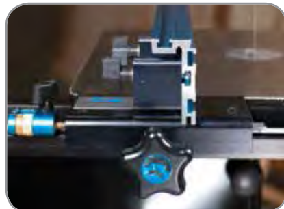
Compensate for blade drift by loosening two hex bolts and adjusting the angle of the fence.
