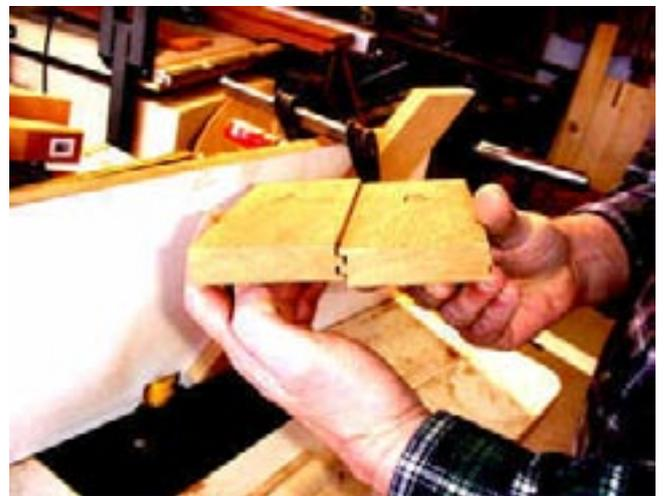
I used the table saw to rip off the first try edges and then raised the router bit several turns (I use a screw adjustment on the router.)
