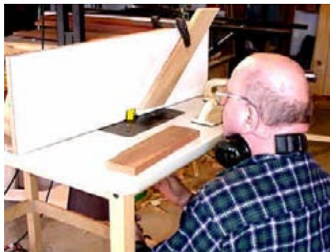
Next, I adjust the fence so that the inside edge of the cut is in line with the fence.
