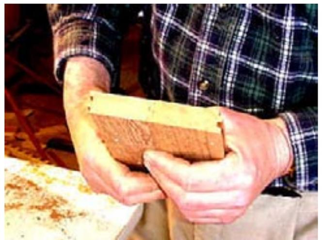
This time, it is right on. So remember, if the “B” side is low, raise the bit. If it is high, lower the bit. Literally, this setup should take no more than a minute or two and it will save you many minutes of planing uneven boards.
