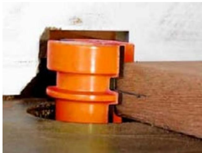
Bit height is the key to success. Any error in height will double the error on the boards you join. It makes real sense to set it right at the beginning.
