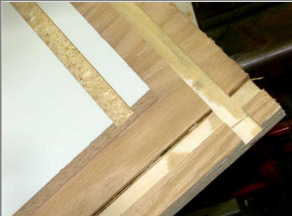
**Here are the cuts she made with the full dado set with chippers to make a 3/4" cut. Joslyn made two cuts in the piece of "cheap" birch plywood. There was no tearout or roughness in the bottoms of the dados. Same with the white melamine particle core board — beautiful clean cuts and a smooth groove. Just think of the beautiful, finished dados she would have when plowing cabinet grade plywood and real wood.**
