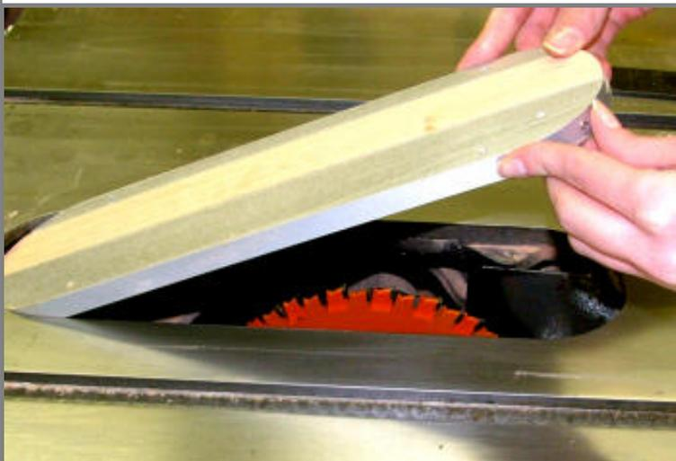
**We will take the time to make zero clearance plates for each of the combinations of blades and chipper sets. Joslyn lowers a blank plate so that she can raise the spinning blades through the wood insert.**
