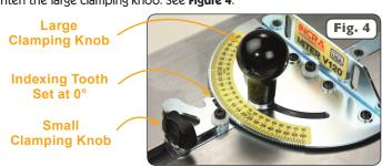
Using the supplied 1/8" hex key, loosen the (4) button head fasteners that secure the faceplate to the protractor and, depending on your application, square the faceplate to the blade, miter slot, sanding belt, etc. **NOTE:** When squaring to a saw blade (see Figure 5), use a reliable square for this important alignment. Securely retighten the (4) button head fasteners to complete the alignment.
