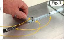
3 Remove the large clamping knob and disengage the indexing tooth from the protractor. Pivot the protractor head to access and adjust the fourth expansion point. See **Figure 3**. Replace the large clamping knob and washer.
