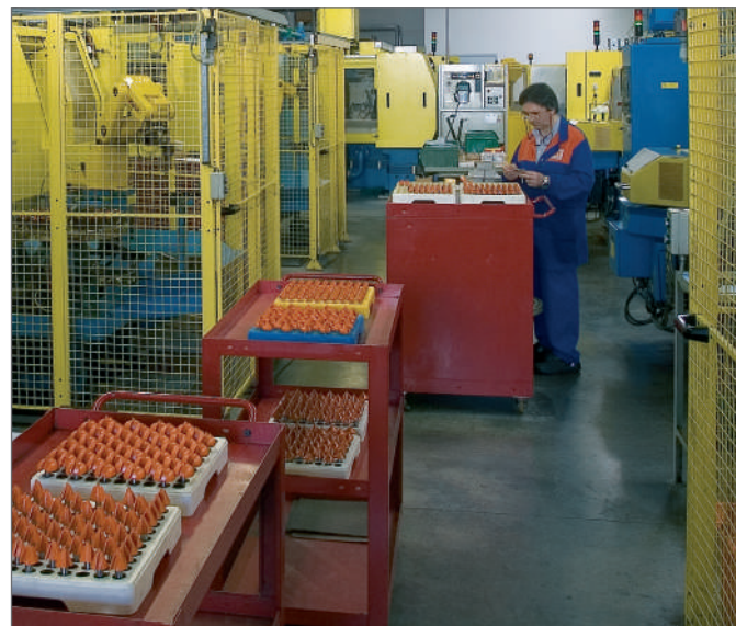
Loading the automated multi-axis CNC sharpening machines.
