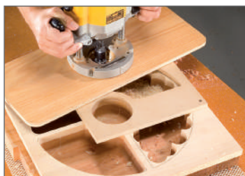
Rout the interior to final shape using the bowl and tray router bit and collet extension.
