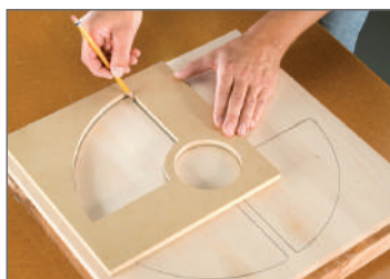
Trace the templates onto the bowl blank.
