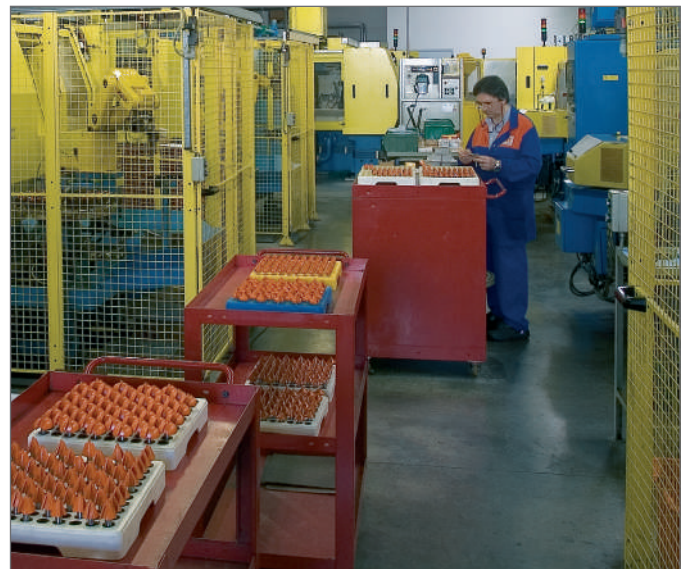
Loading the automated multi-axis CNC sharpening machines.
