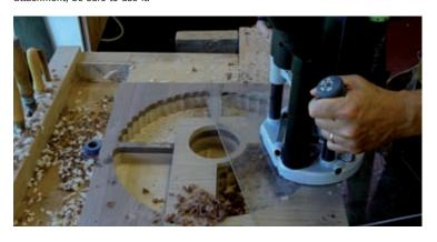
Secure the blank to your bench. With the plunge mechanism set at the top of its travel, place the router over an open area on the template. Make sure the cutter is not contacting the wood and turn on the router. Gently slide the router to the template edge and begin your cut. Continue the cut around the opening.
