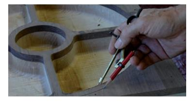
The next step is to lay out the outside wall of the bowl. Set a compass to mark a little over 12,7mm to allow for sanding. Make sure the compass point extends about 6,35mm or so past the pencil point.
