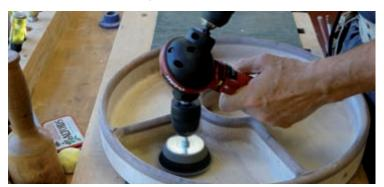
Sand the interior of the bowl using a soft disc. These discs are commonly used by lathe turners on lathe-turned bowl interiors. Start with 80-grit and work your way up to 220-grit. Finish sanding the outside with an orbital sander. Now you're ready to apply a finish. A great food safe finish for wood is walnut oil. You'll find it at most health food stores. It dries hard and is totally non-toxic. Other food safe finishes include mineral oil, salad bowl finish and shellac.
