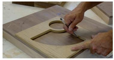
Lay out the bowl using the template. Center the template on the blank and mark the first partition. Remove the template and make marks exactly 12,7mm from the edge of the first partition. This defines the wall thickness for each partition. It's important to be exact in order to achieve a uniform wall thickness for all the partitions. Use these marks to align the template for the two adjoining partitions. Make additional marks to position the template for the last partition.
