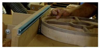
With the bowl sanded round and the band saw marks removed, head to the router table for some final shaping. Mount a 12,7mm roundover bit in the router and round over the bottom edge of the bowl.
