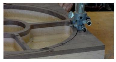
Take the blank to the bandsaw and cut off the excess stock. Take care to cut up to the layout line. Go slowly and do your best to make the cut smooth and accurate. It'll save you a lot of sanding later.
