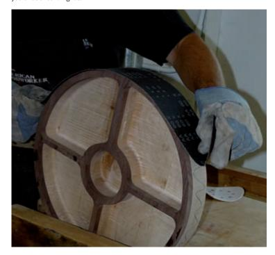
The bowl will come off the band saw round but rough. Sand the band sawn edge smooth and fair. A good way to sand the edge on a round bowl is to use a sanding belt. Pencil marks on the outside edge tell you where the low spots are and where you've sanded. Clamp the bowl blank in a vise (use scrap wood to protect the bowl form iron jaws) and sand the edge like a shoeshine polishes a shoe.
