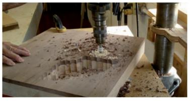
Use a Forstner bit in a drill press to remove most of the wood. Forstner bits do the best job because they can make overlapping cuts and leave a flat bottom.
